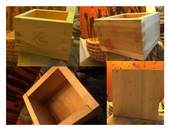
I drilled 26 holes in the bottom of the box. Seems like a lot now that I look at the pictures. Maybe being in the club has revealed some anger issues, not sure. I sanded for about 2 days straight. I bought special round files to smooth the inside of the drainage holes. Research brought me to Minwax Polycrylic as e sealant that would least affect the natural wood look of the cup.
